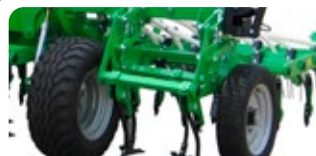
SNP-4 wing floating system and depth control wheels
