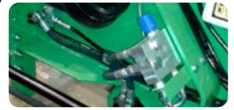
Flow regulation kit for the unloading endless screw RT 65 *Only for tractor with oil flow superior to 60 L/m that cannot be regulated.
