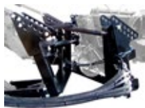
Lateral movement of box and vibrating head
