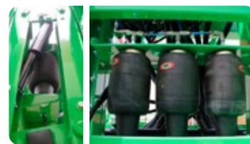
Reinforced air suspension S3 and S4 depending boom model.
