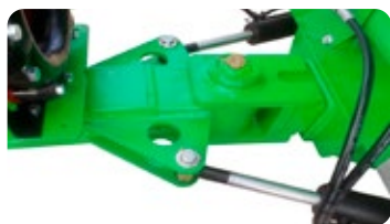
Articulated directional lance with 2 hydraulic cylinders.
